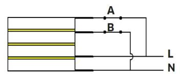
Alternative power output of the element when connected to a power supply:
