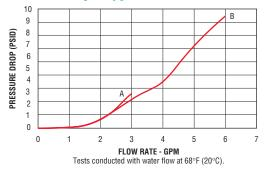
Flow Range A .53 - 2.1 GPM 2 - 8 LPM Flow Range B .79 - 6.6 GPM 3 - 25 LPM
