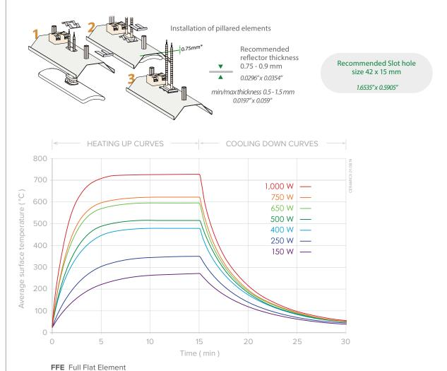
Heating up and cooling down curves showing average surface temperature taken with an infrared thermometer set at an emissivity of 0.95 (Element mounted in an aluminised steel reflector RAS)
