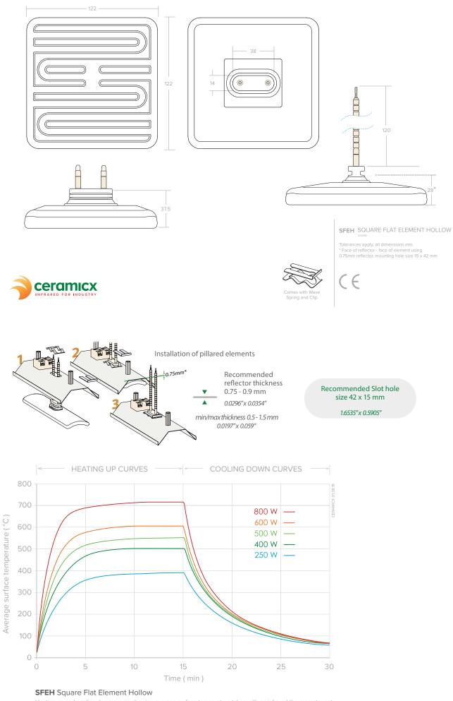
Heating up and cooling down curves showing average surface temperature taken with an infrared thermometer set at an emissivity of 0.95 (Element mounted in an aluminised steel reflector RAS)
