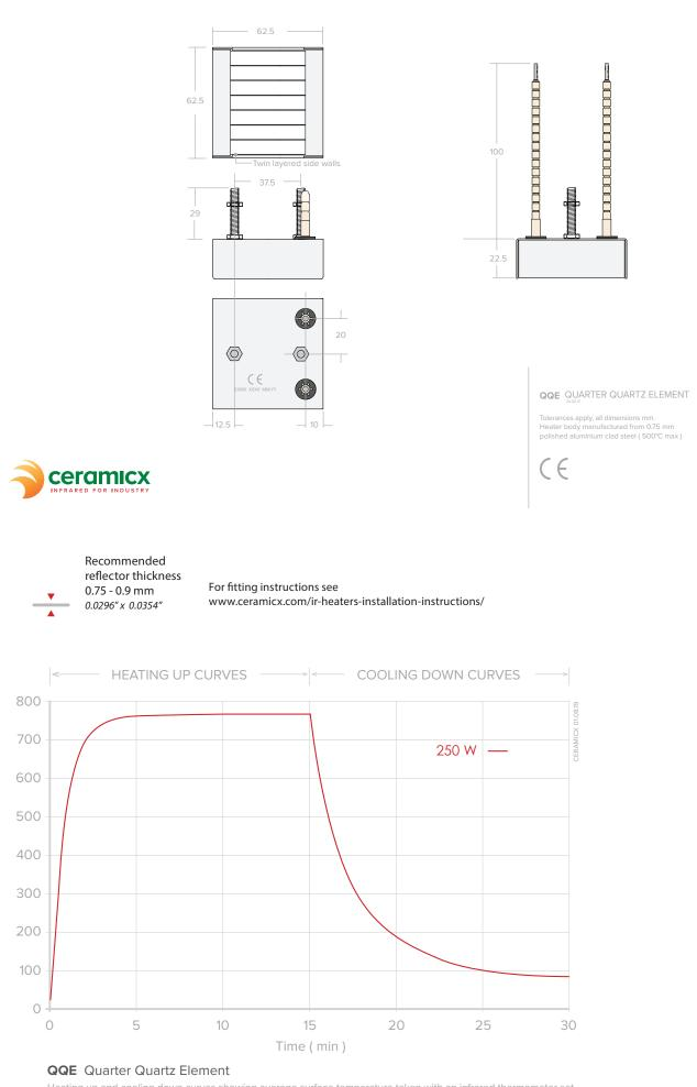
Heating up and cooling down curves showing average surface temperature taken with an infrared thermometer set at an emissivity of 0.7
