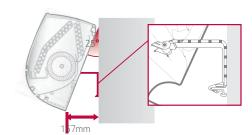
Detachable Bottom Cover The air conditioner's bottom cover is detachable for easier installation and access.
