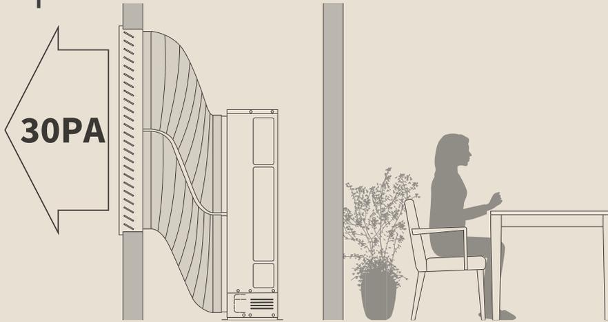
Thanks to the external static pressure now available, our SET FREE Mini units can be installed inside a plant room while preserving the aesthetics of your buildings.
